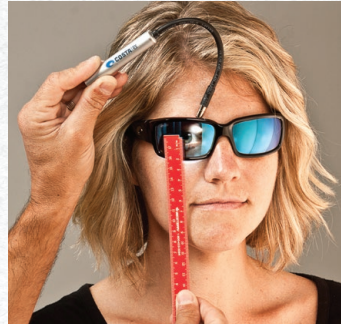
ILLUMINATING THE BACK OF THE LENS WITH THE COSTA SEG SNAKE LETS YOU EASILY SEE THE PUPIL AND EYELID.
